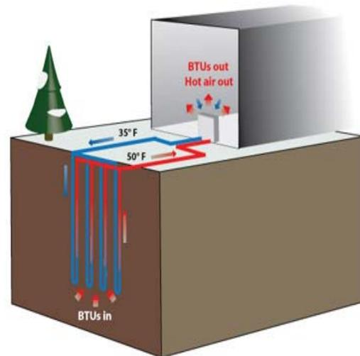
heat from inside into hot outside air, the pump transfers it to a fluid (a water and glycol mix) and circulates it through pipes that are buried in the ground. That requires a lot less electricity.
